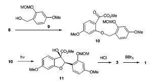
transformation of **3** into coumestrol was achieved in 75% yield using 10 equiv of BBr<sub>3</sub> in methylene chloride from -78 °C to 25 °C for 12 h.<sup>11</sup> The proton NMR spectrum of this compound was identical to the NMR of an authentic sample.<sup>12</sup>
